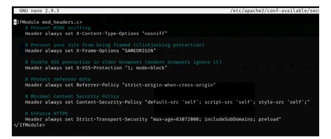
Enable the security headers: **sudo a2enconf security-headers** Restart Apache to apply changes: **sudo systemctl reload apache2**
